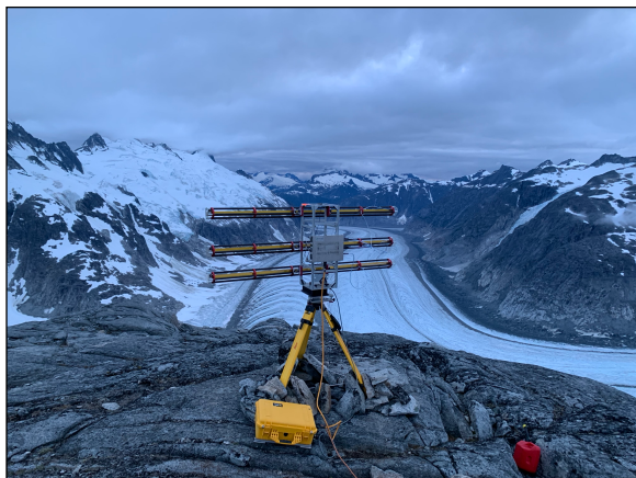
Fig. 1. Gamma Terrestrial Radar Interferometer viewing the Juneau Icefield to capture movement and spatial-temporal variations in surface melt.
