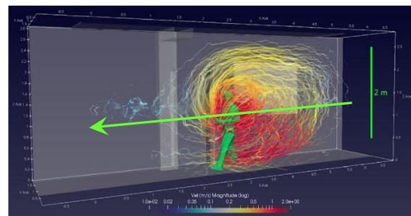
**Figure 1.**  $5.2 \times 10^{13}$  particle interactions simulate the displacement of air (visualized as streamlines) after a figure moves through the hallway, from right to left. Warmer colors represent greater velocity magnitude.
