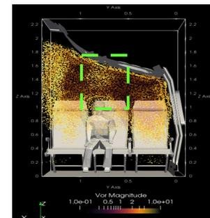
**Figure 2.** A 3D model of a gasper jet in an airplane passenger cabin. The use of gaspers is likely to be an effective personal defense strategy by enforcing an exclusive region of filtered air across a person's face.
