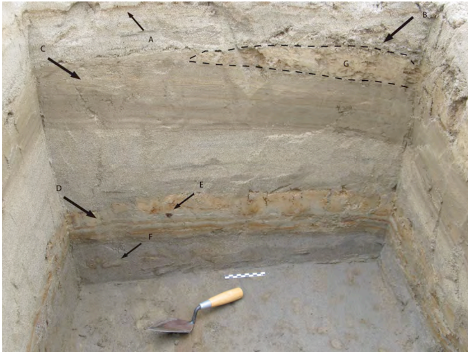
Figure 9: Test Pit 43 A) thin clay lens B) salt concretions C) interlaminated sand and clay D) rhythmites of oxidized and unoxidized clays E) dark red organic remains F) semi-circular iron-oxide staining G) Clay wedge
