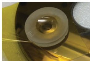
Fig. 1. Single-opening epoxy mounts, polished on each side for flatness, adhered to specially formulated tape and a super flat hard drive surface.
