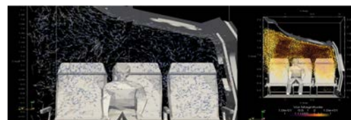
Figure 2. Turbulent airflow in an airplane cabin.
