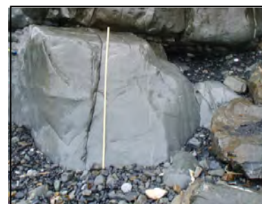
Fig. 2. Non-Fault damaged bedrock with high cohesion.
