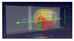
**Figure 1**. 5.2\*10<sup>13</sup> particle interactions simulate the displacement of air (visualized as streamlines) after a figure moves through the hallway, from right to left. Warmer colors represent greater velocity magnitude.
